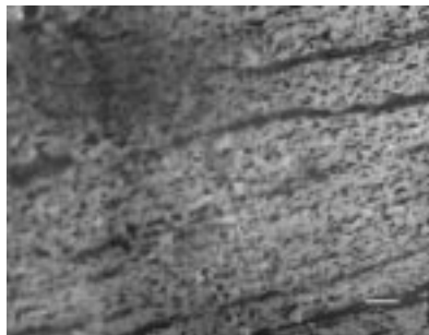
Fig. 6 Micrographic aspect of Y-123 sample with Ag(In) 7.5 wt% and Y-211 30 wt% melt processed at 1170°C. The marker represents 100 \mu
