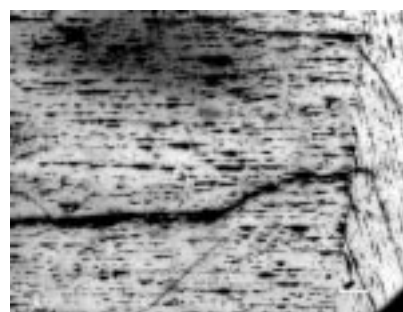
Fig. 3b Micrographic aspect of Y-123 sample with Ag 7.5 wt% and Y-211 30 wt% melt processed at 1170°C. The marker represents 100 \mu
